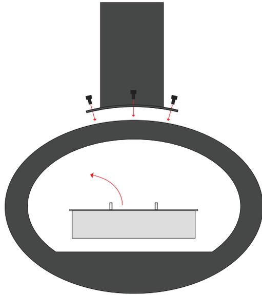
Remove the burner from the fireplace, to avoid damage to the fireplace during installation.
