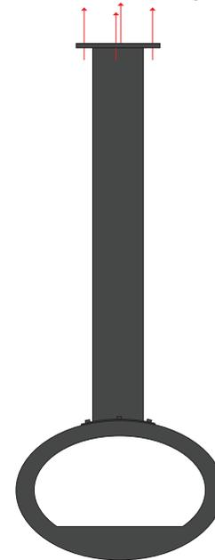
Attach the fireplace to the ceiling, using 4 appropriate screws and plugs, which are compatible with your ceiling.
